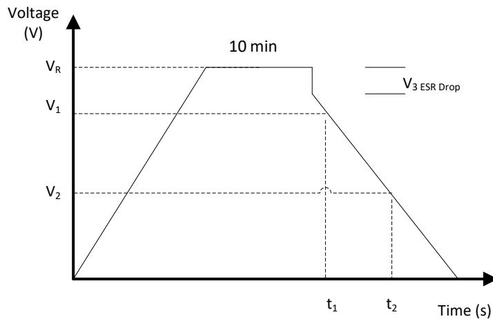
$I$  – Discharge Current,  $4 \times C \times V_R$  (mA)
