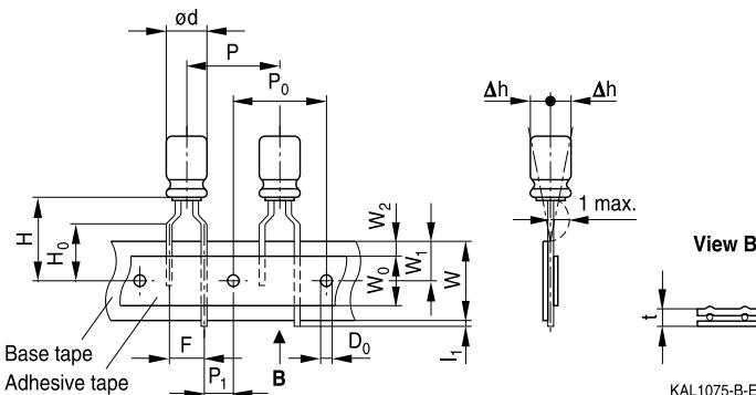
**Lead spacing 5.0 mm ( $\varnothing d = 10 \dots 12.5 \text{ mm}$ )**
