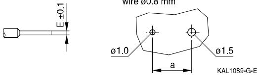
**Suggestion for PCB hole diameter, wire  $\varnothing 1.0$  mm**
