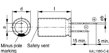
Safety vent for diameter  $\geq 6.3$  mm.
