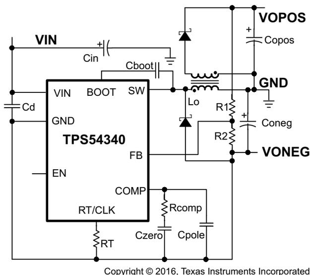
**Figure 51. TPS54340 Split Rail Power Supply**
