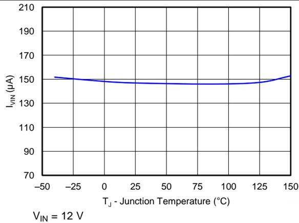
Figure 17.  $V_{IN}$  Supply Current vs Junction Temperature
