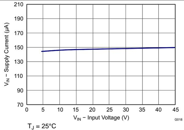
Figure 18.  $V_{IN}$  Supply Current vs Input Voltage
