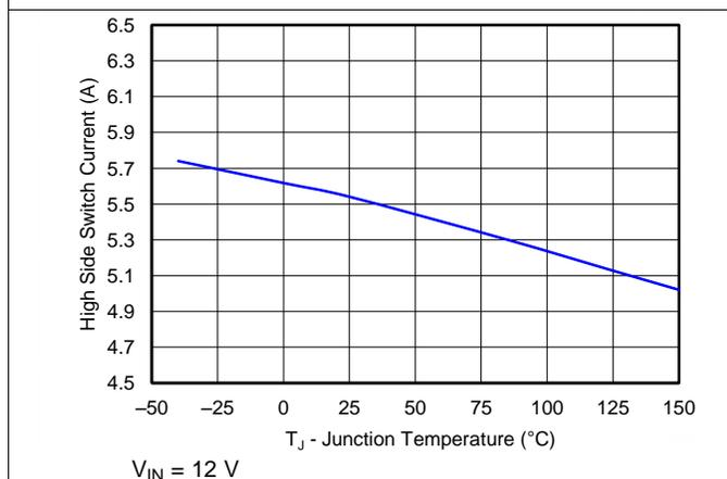
Figure 3. Switch Current Limit vs Junction Temperature
