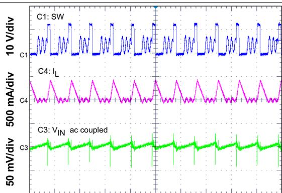
Figure 41. Input Ripple DCM
