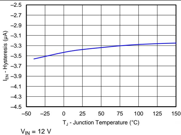
Figure 13. EN Terminal Current Hysteresis vs Junction Temperature
