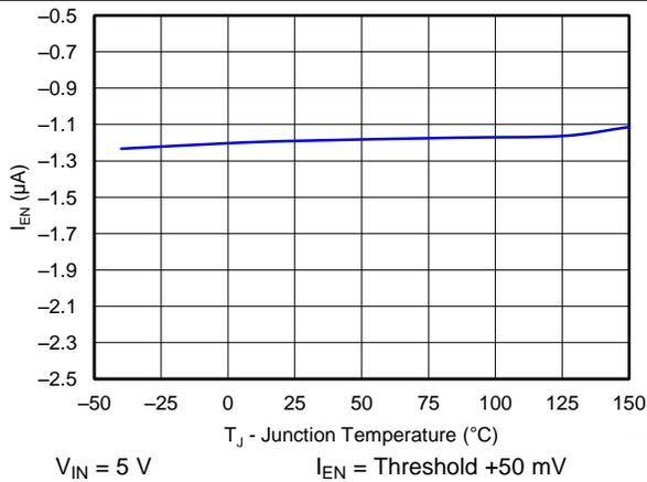
Figure 11. EN Terminal Current vs Junction Temperature
