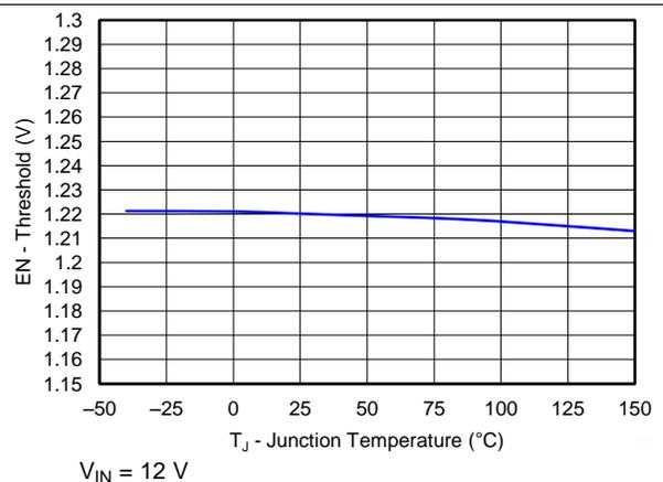
Figure 10. EN Terminal Voltage vs Junction Temperature
