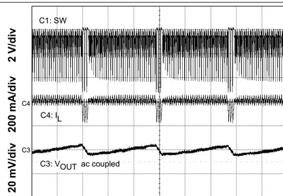
Figure 42. Low Dropout Operation
