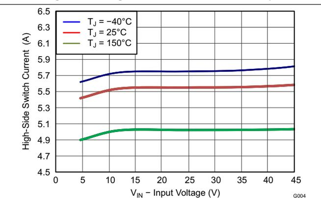
Figure 4. Switch Current Limit vs Input Voltage
