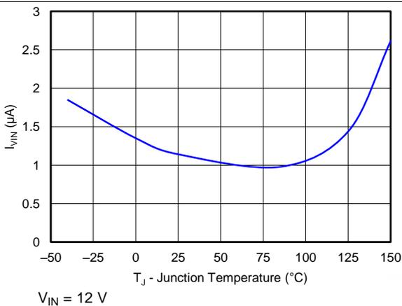
Figure 15. Shutdown Supply Current vs Junction Temperature
