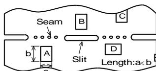
Products (A,B,C,D) shall be located carefully so that products are not subject to the mechanical stress due to warping the board. Because they may be subjected the mechanical stress in order of A>C>B≠D.
