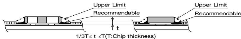
Accordingly increasing the solder volume, the mechanical stress to product is also increased.
