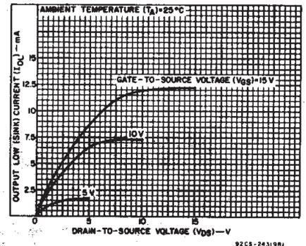
Fig. 6 - Minimum output low (sink) current characteristics.
