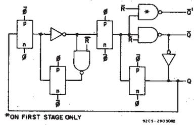
Fig. 4 - Detail of typical flip-flop stage.
