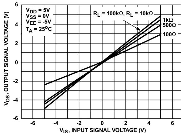
Figure 30. ON Characteristics for 1 of 8 Channels (CD4051B)
