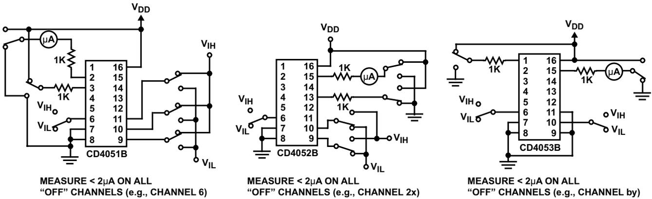
Figure 17. Input Voltage Test Circuits (Noise Immunity)
