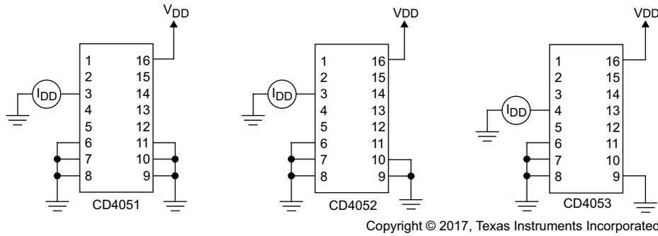
**Figure 13. On Channel Leakage Current - Any Channel On**
