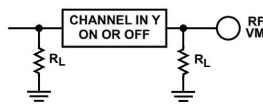
Figure 23. Crosstalk Between Duals or Triplets (CD4052B, CD4053B)
