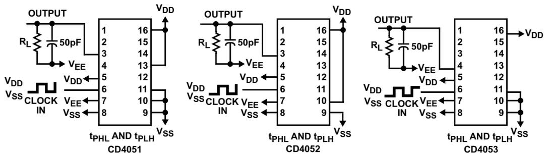
**Figure 16. Propagation Delay - Inhibit Input to Signal Output**
