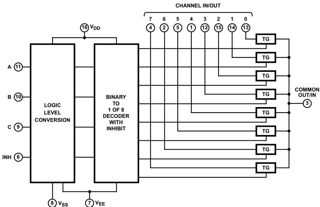
All inputs are protected by standard CMOS protection network.
