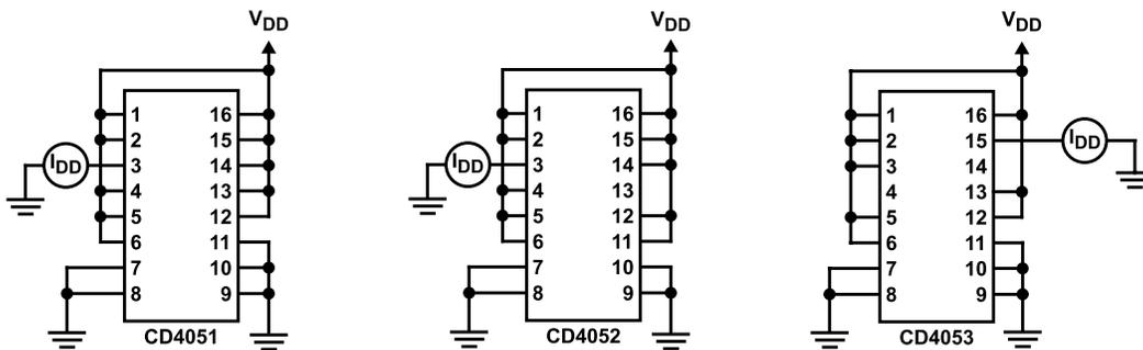
**Figure 14. OFF Channel Leakage Current - All Channels OFF**
