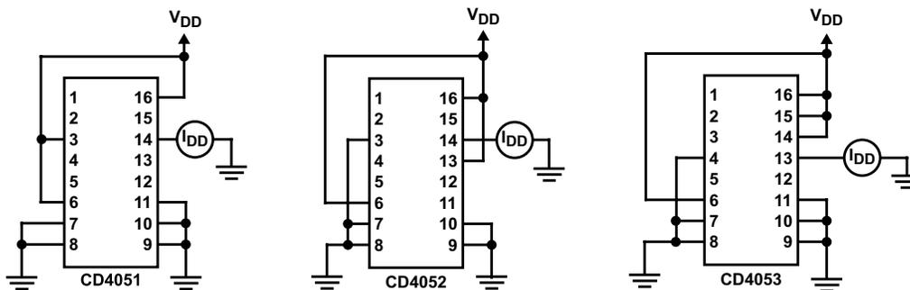
Figure 12. OFF Channel Leakage Current - Any Channel OFF
