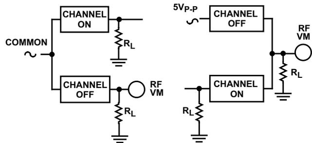
Figure 22. Crosstalk Between Any Two Channels (All Types)
