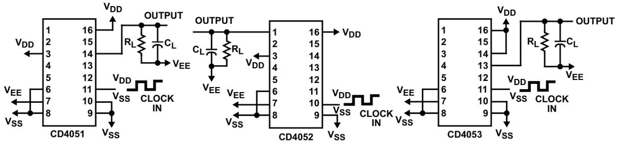
**Figure 15. Propagation Delay - Address Input to Signal Output**
