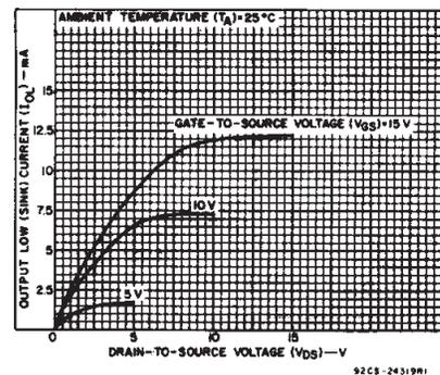
Fig. 4 - Minimum output low (sink) current characteristics.
