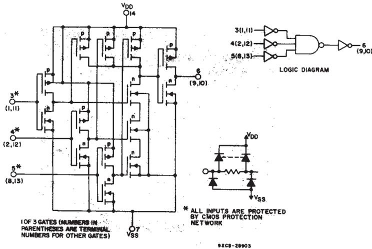
Fig.7 - Schematic and logic diagrams for CD4025B.
