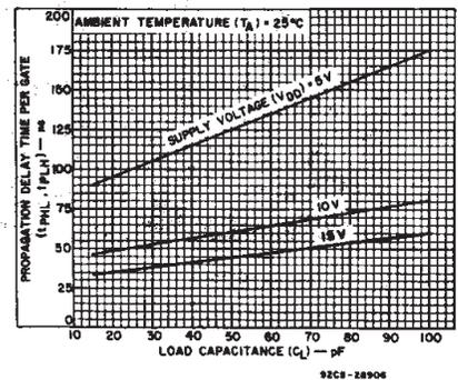
Fig.11 - Typical propagation delay time vs. load capacitance.
