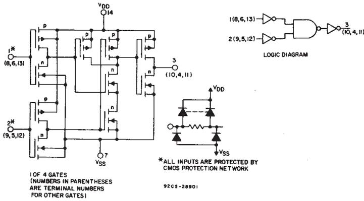
Fig.5 - Schematic and logic diagrams for CD4001B.
