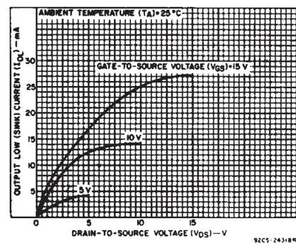
Fig. 3 - Typical output low (sink) current characteristics.
