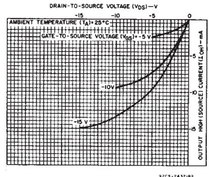
Fig.9 - Minimum output high (source) current characteristics.
