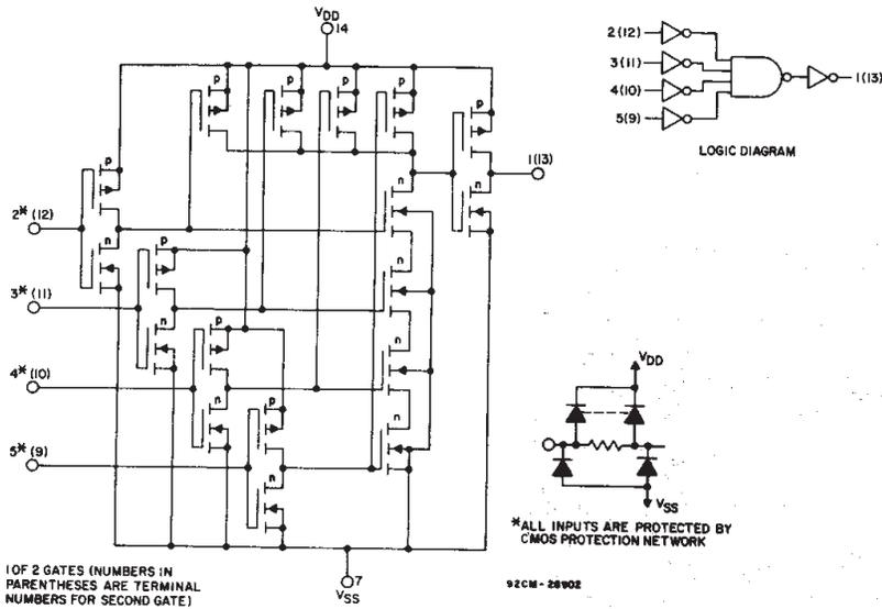
Fig.6 - Schematic and logic diagrams for CD4002B.
