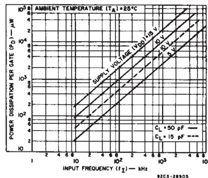
Fig. 2 - Typical power dissipation vs. frequency.
