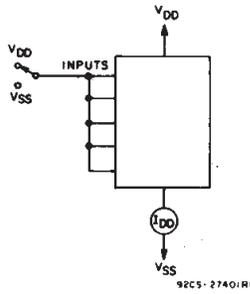
Fig. 10 - Quiescent device current test circuit.
