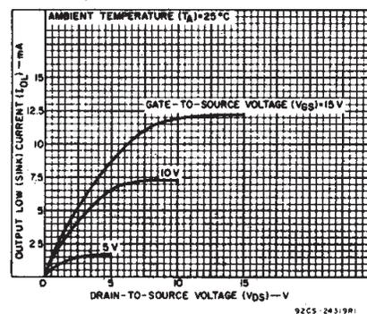
Fig. 3 - Minimum output low (sink) current characteristics.
