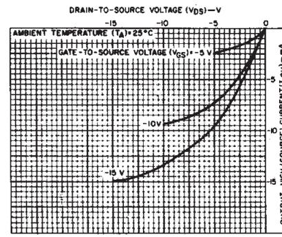
Fig. 5 - Minimum output high (source) current characteristics.
