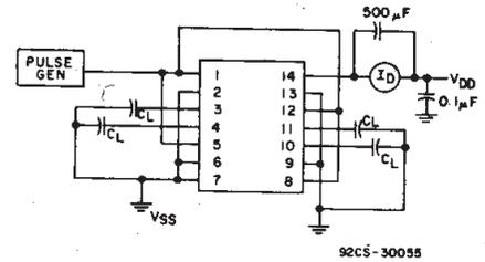
Fig. 13 - Dynamic power dissipation test circuit.
