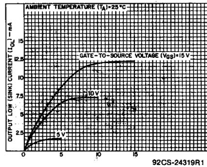
Fig. 5 - Minimum output low (sink) current characteristics.
