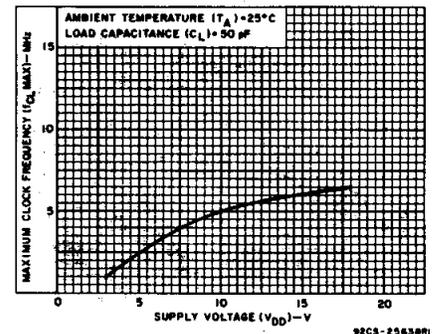
Fig. 15 - Typical maximum-clock-frequency vs. supply voltage.
