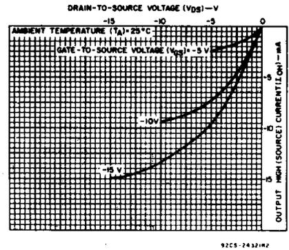
Fig. 7 - Minimum output high (source) current characteristics.
