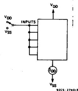
Fig. 17 — Quiescent device current test circuit.
