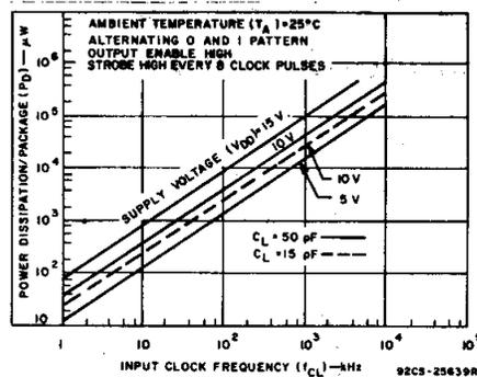
Fig. 16 — Dynamic power dissipation vs input clock frequency.
