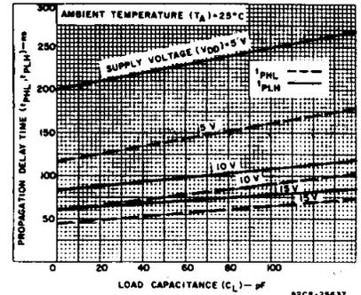
Fig. 12 - Output enable-to-parallel output propagation delay vs. C<sub>L</sub>.
