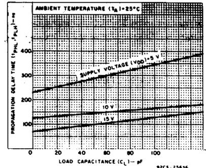
Fig. 11 - Strobe-to-parallel output propagation delay vs. C<sub>L</sub>.
