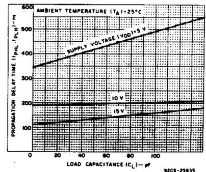
Fig. 10 - Clock-to-parallel output propagation delay vs  $C_L$ .
