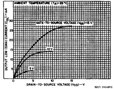
Fig. 4 - Typical output low (sink) current characteristics.
