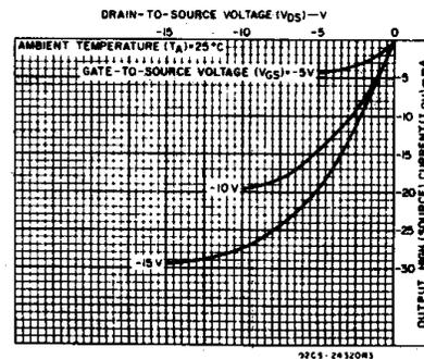
Fig. 8 - Typical output high (source) current characteristics.
