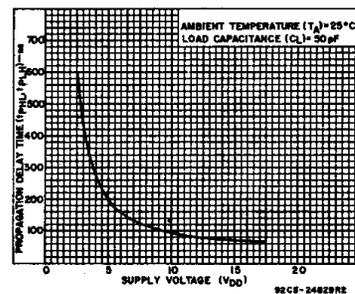
Fig. 10 - Typical propagation delay time vs. supply voltage.
