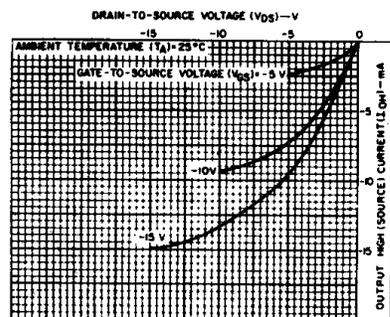
Fig. 9 - Minimum output high (source) current characteristics.
