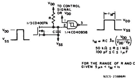
Fig. 17 - Monostable multivibrator.
