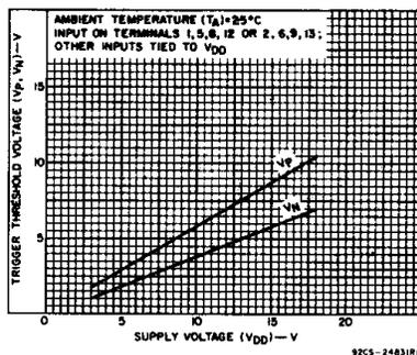
Fig. 12 - Typical trigger threshold voltage vs. V<sub>DD</sub>
