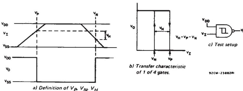
Fig. 2 – Hysteresis definition, characteristic, and test setup.
