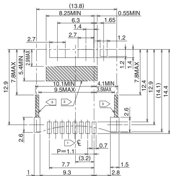
Note 1  $\phi$  indicates the center line of the microSD card slot.
