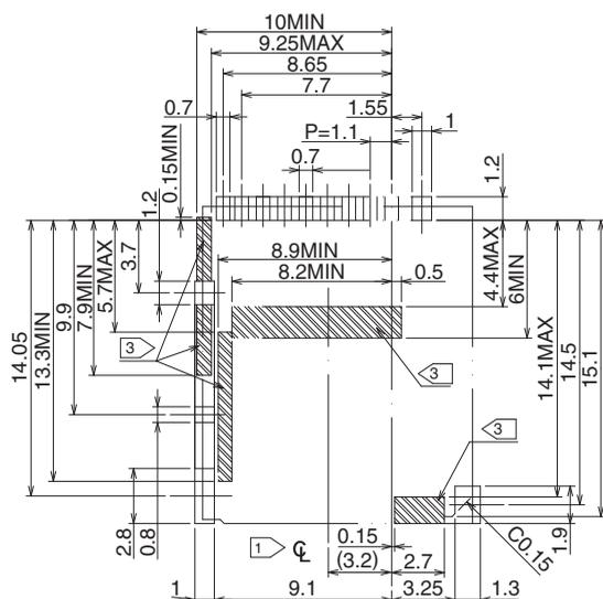
Note 1  $\phi$  indicates the center line of the microSD card slot.
