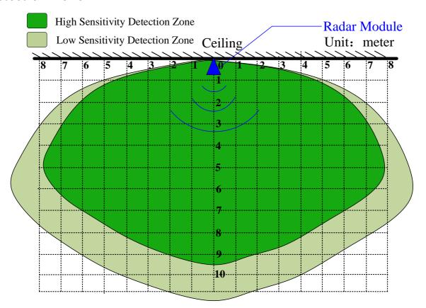
Figure 4 BPS1818-A1 Detection Pattern
