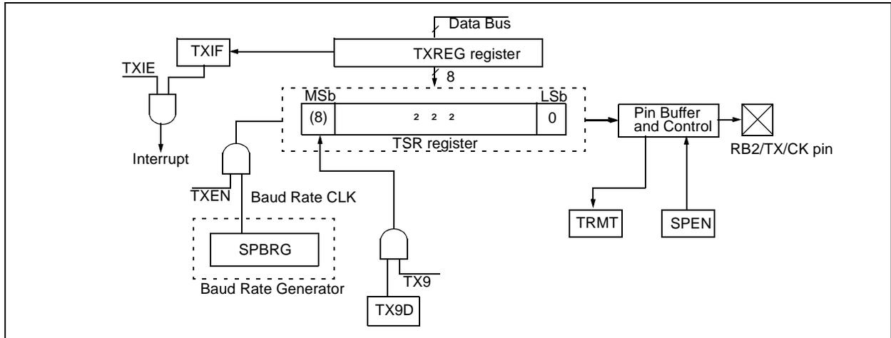
Follow these steps when setting up an Asynchronous Transmission:
