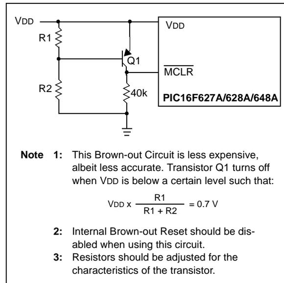
**FIGURE 14-12: EXTERNAL BROWN-OUT PROTECTION CIRCUIT 1**
