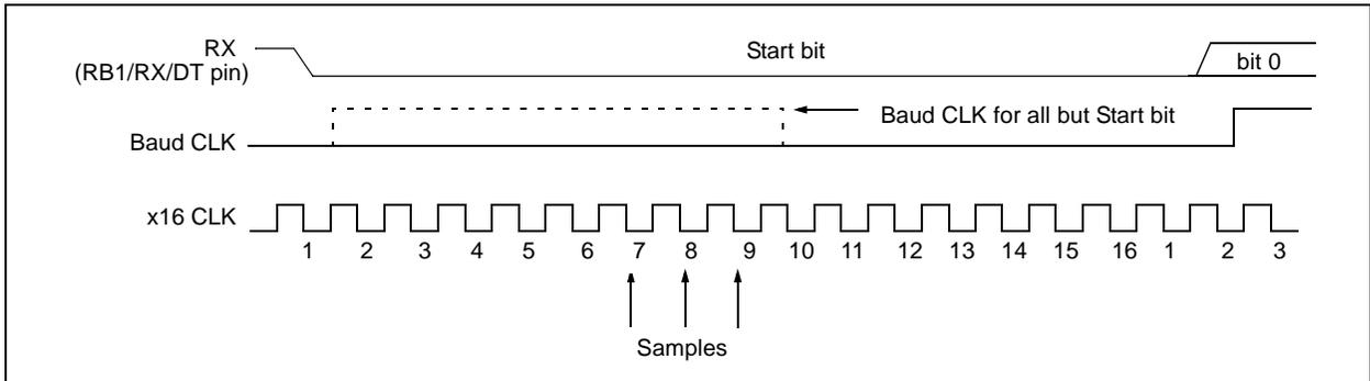
**FIGURE 12-2: RX PIN SAMPLING SCHEME, BRGH = 1**
