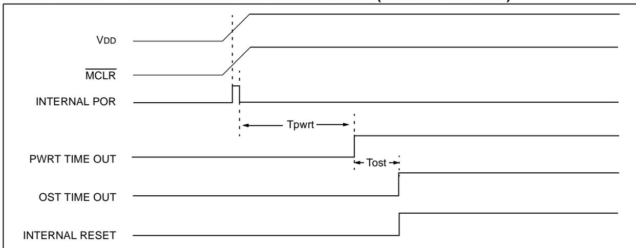
**FIGURE 14-11: EXTERNAL POWER-ON RESET CIRCUIT (FOR SLOW V<sub>DD</sub> POWER-UP)**
