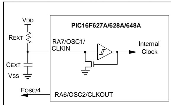
The RC Oscillator mode has two options that control the unused OSC2 pin. The first allows it to be used as a general purpose I/O port. The other configures the pin as an output providing the F<sub>osc</sub> signal (internal clock divided by 4) for test or external synchronization purposes.
