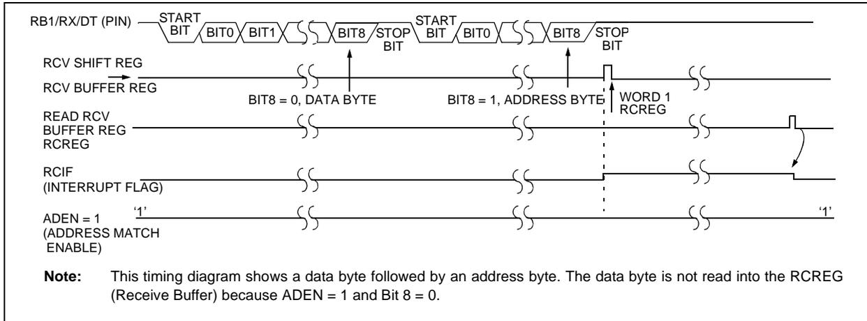
**FIGURE 12-10: ASYNCHRONOUS RECEPTION WITH ADDRESS BYTE FIRST**
