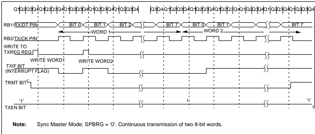
**FIGURE 12-13: SYNCHRONOUS TRANSMISSION (THROUGH TXEN)**
