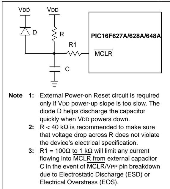
**FIGURE 14-13: EXTERNAL BROWN-OUT PROTECTION CIRCUIT 2**
