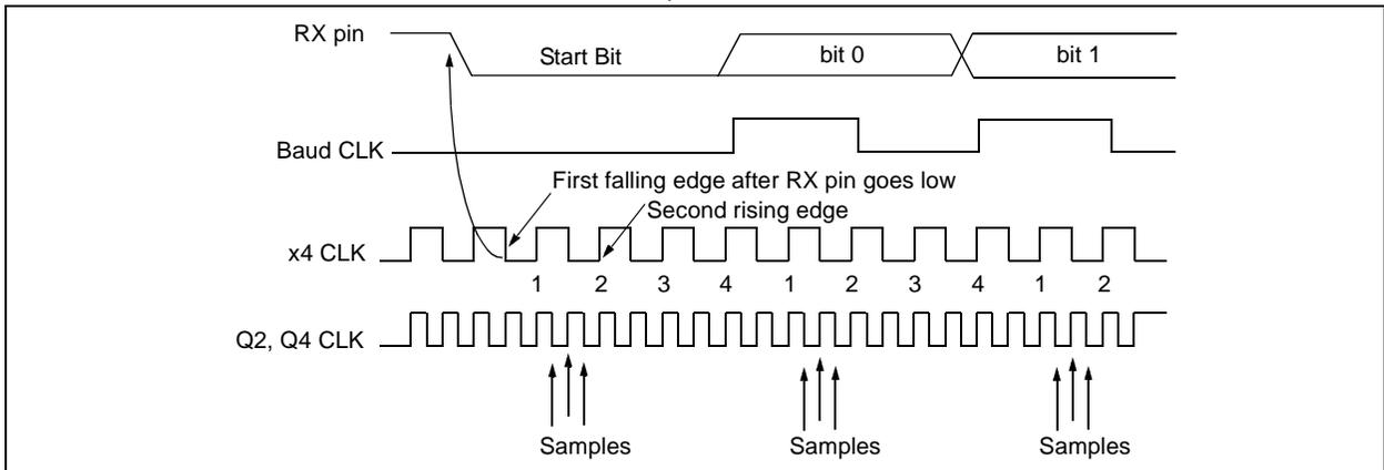
**FIGURE 12-3: RX PIN SAMPLING SCHEME, BRGH = 1**
