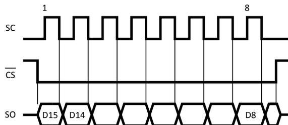
Figure 10. Reading Continuous Conversion - Single Eight-Bit Frame
