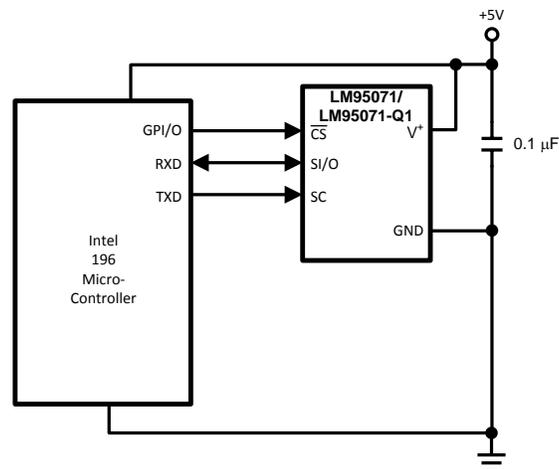
Figure 14. Temperature monitor using Intel 196 processor
