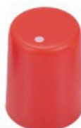
46135 Rotary knob with light texture Material: ABS Diameter: 12.9 mm Height: 15 mm Shaft hole: 6 x 4.5 mm
