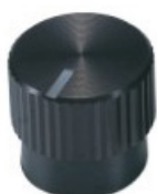
46105 Aluminum shell knob with ABS plastic insert straight knurl and indicator line on top
