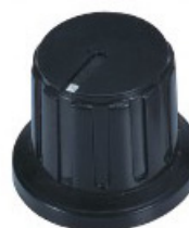
46136 Fluted plastic knob with square indicator on top, gloss finish Material: ABS Diameter: 20 mm Height: 14.9 mm Shaft hole: \varnothing 6 mm, 18 Teeth
