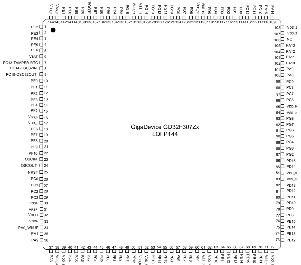
Figure 2-2 GD32F307Zx LQFP144 pinouts
